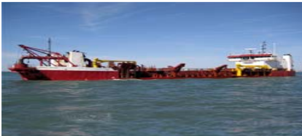
The Padre Island, one of two hopper dredgers to be used on the project
