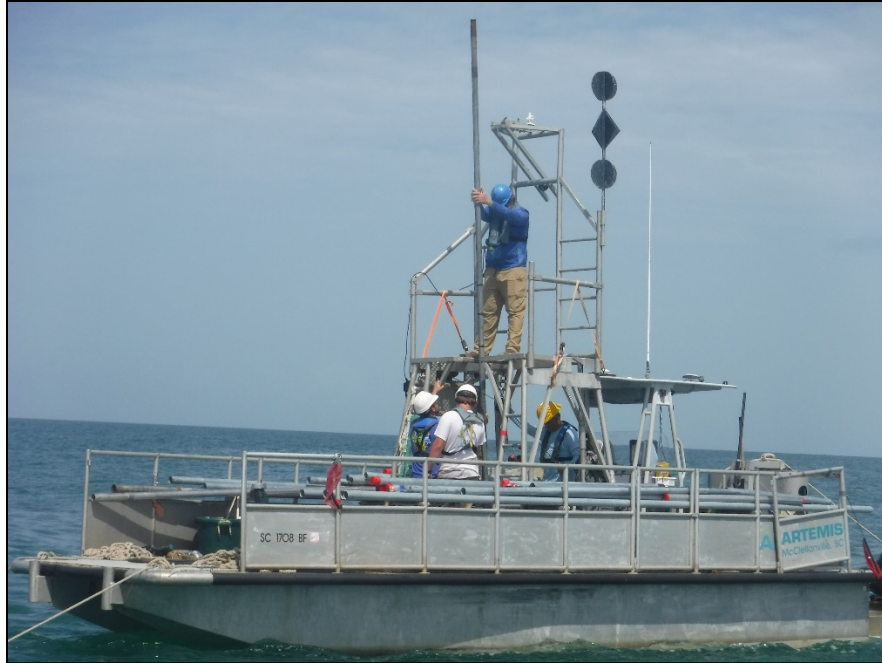
Figure 17. Athena vibracores collection aboard the RV Artemis .
